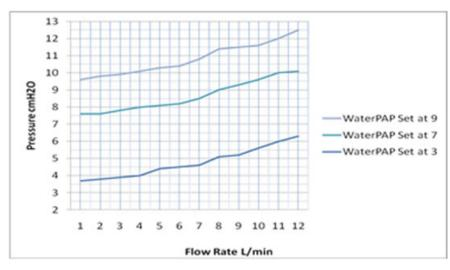
This data was generated using a standard 10mm heated ventilator circuit. Results may vary depending on the type and length of the circuit being used.
