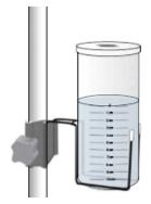
Fill the canister with water to the 0 cm line
